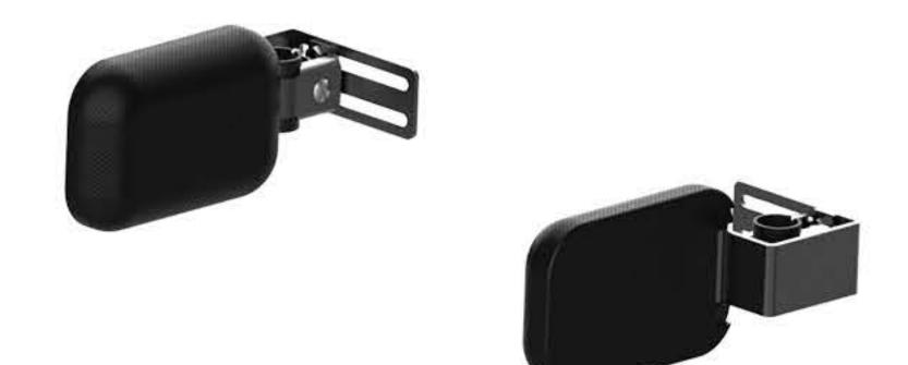
These lateral trunk supports bolt on to the back canes. Each pad is adjustable for depth, angle, height and width. The pads have a 4 x 5 array of holes on the back. Each pad includes a washable fabric cover.
